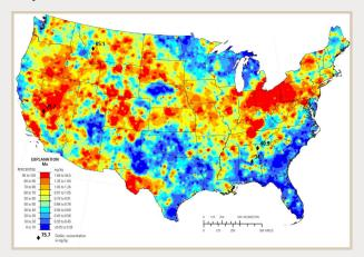
This map, adapted from a U.S. Geological Survey (USGS) report, <sup>3</sup> shows relative amounts of naturally occurring molybdenum in surface soils across the United States. The USGS data shows that national average molybdenum concentration in surface soils in the U.S. is approximately 1 mg/kg<sup>4</sup> but can range much higher in some areas of the country.
